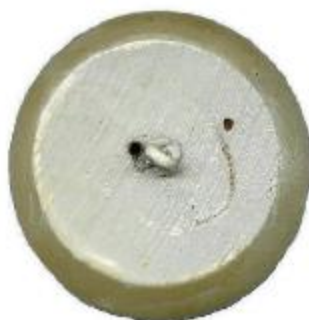
NOTE SAW/GRINDING MARKS, VERTICAL HOLE & BUBBLE
